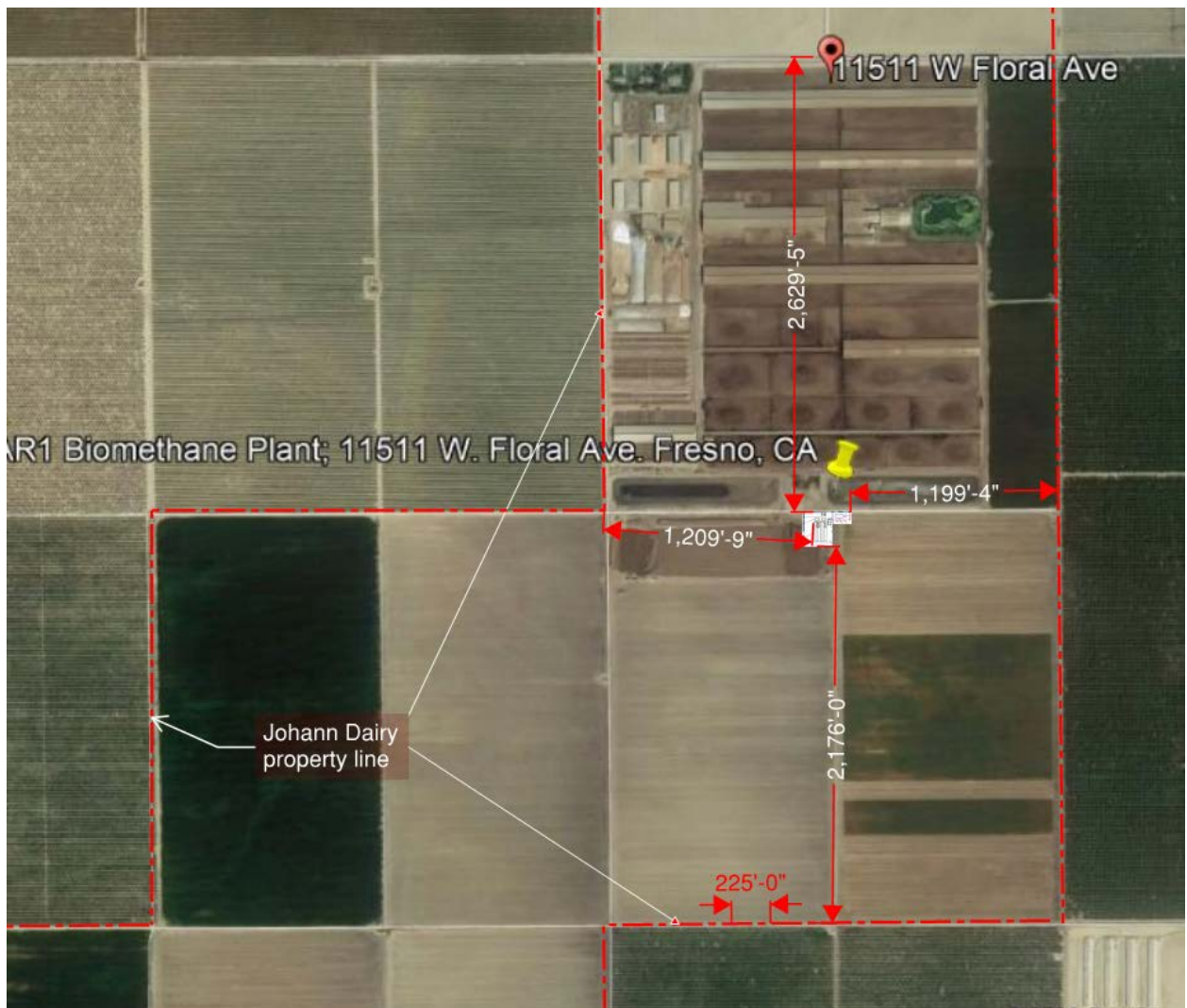
Figure 2: Portion of Johann Dairy Property to show SAR1 Project setbacks from property boundary
