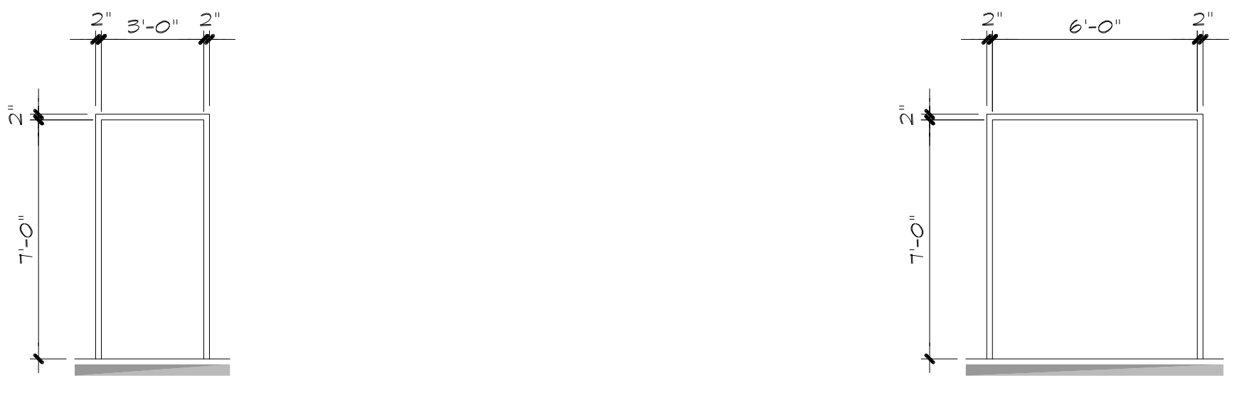
1 HM SINGLE DOOR 2 ALUMINUM STOREFRONT SYSTEM, SEE WINDOW ELEVATIONS. 3 HM DOUBLE DOOR
