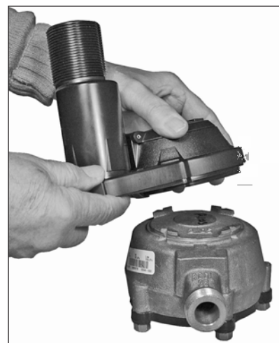
Figure 45: Remove assembly from meter
