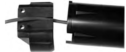
Figure 18: Threading cable harness
