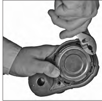
Figure 46: Pull tab to remove the breakaway plate
