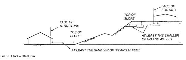
FIGURE 1808A.7.1 FOUNDATION CLEARANCES FROM SLOPES **1808A.8 Concrete foundations.** The design, materials and construction of concrete foundations shall comply with Sections 1808A.8.1 through 1808A.8.6 and the provisions of Chapter 19A.
