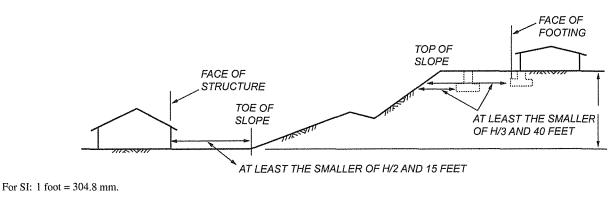
FIGURE 1808.7.1 FOUNDATION CLEARANCES FROM SLOPES
